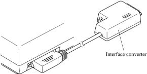
Plug one end of a serial cable into the serial interface connector's 25-pin D-TYPE connector.
