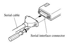
☐ Plug the other end of the serial cable into your computer's serial ports. Serial ports are usually marked COM1, COM 2, etc. If your computer has only one serial port, it will be marked COM1.
