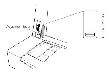
Unlock the tractor on the left (when viewing the printer from behind) by pulling its gray lever up, and adjust the position of the left tractor.
