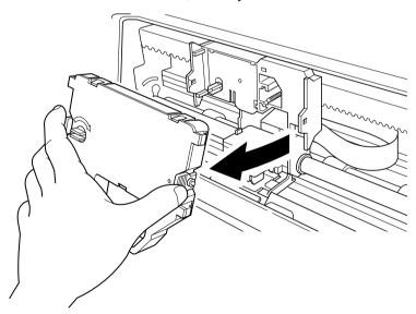
Use the procedure under "Installing the ribbon cassette" on page 5 to install a new cassette.
