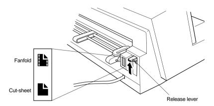
☐ Set the adjustment lever to the value that matches the thickness of the paper you are using. The setting for normal paper is 1. Set the lever to a larger value for thicker paper, or to a smaller value for thinner paper. See the table on page 58 for details.
